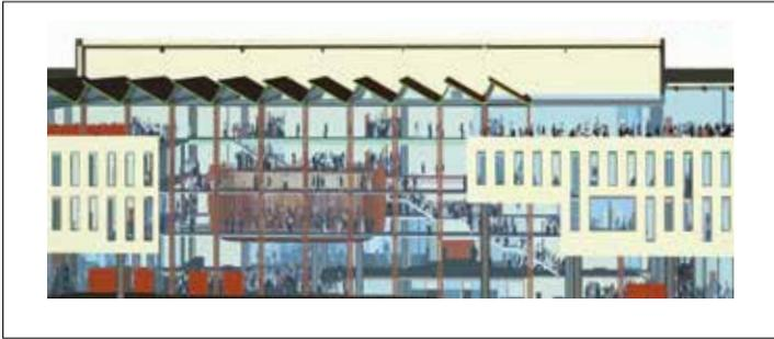
*A human movement simulator program is used to analyse the timed exit information along with the spatial geometries for the building, like the number and location of exits, and data on fire and smoke behavior from the computational fluid dynamics (CFD) model. The program models occupant movement in different fire scenarios, specific to the building design and user population, and determines egress time.*
