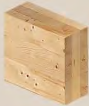
Cross Laminated Timber Used for floor slabs
