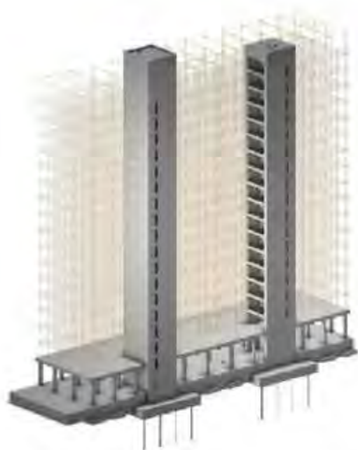
Cast-In-Place Reinforced Concrete Structure
