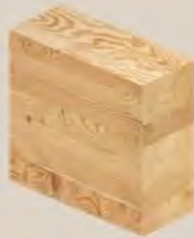
Glue Laminated Timber Used for structural columns
