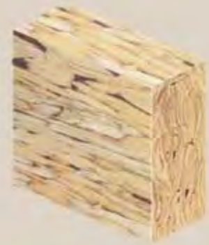
Parallel Strand Lumber Used for heavy-loaded structural columns
