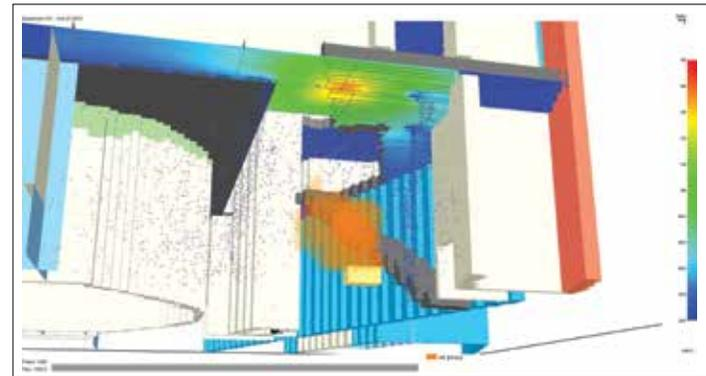
*A computational fluid dynamics (CFD) modelling program simulates and assesses the behavior of fire and smoke, as well as the temperature of interior spaces and building components. The calculations include information on the effects of both the passive aspects of the building (such as the shapes of the spaces and types of materials) and the active systems (such as sprinklers and smoke management systems).*
