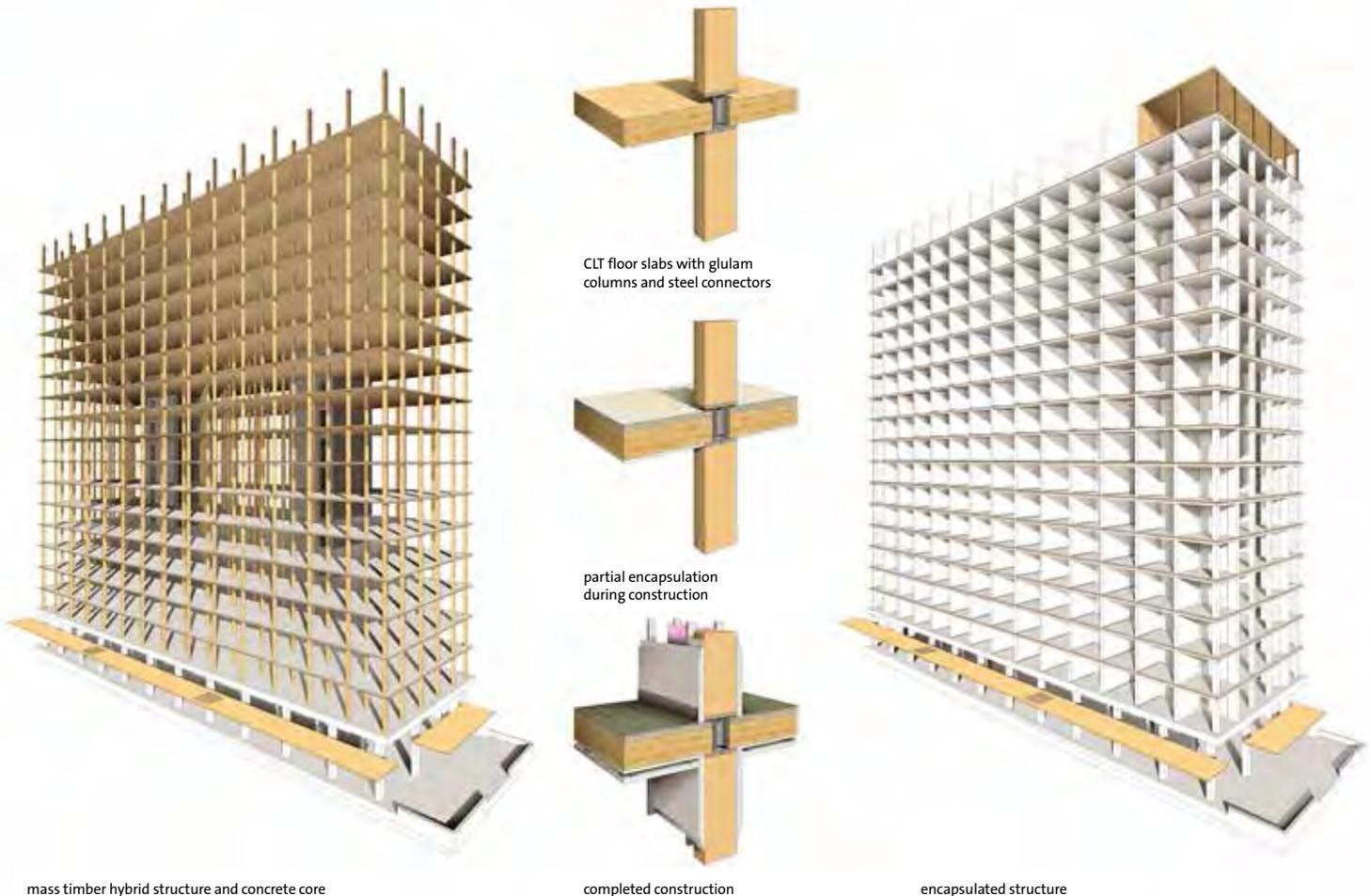
*The overall simplicity of the design of Brock Commons is broadly recognized as being key to the affordability, safety and efficient construction of the building.*
